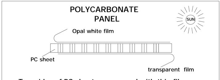
Two sides of PC sheet are covered with thin film, one side's film is transparent, another's film is opal white. The UV-protected side of the sheet is covered with opal white film and must face towards the sun.
