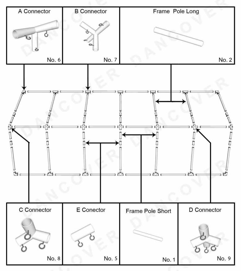
Step 1: Lay out all roof tubes and connectors as shown above.
