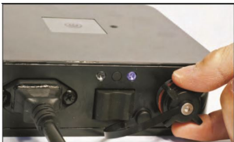
5.1 Unscrew the cap next to the switch.
