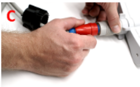
Push the sleeve to the end.
