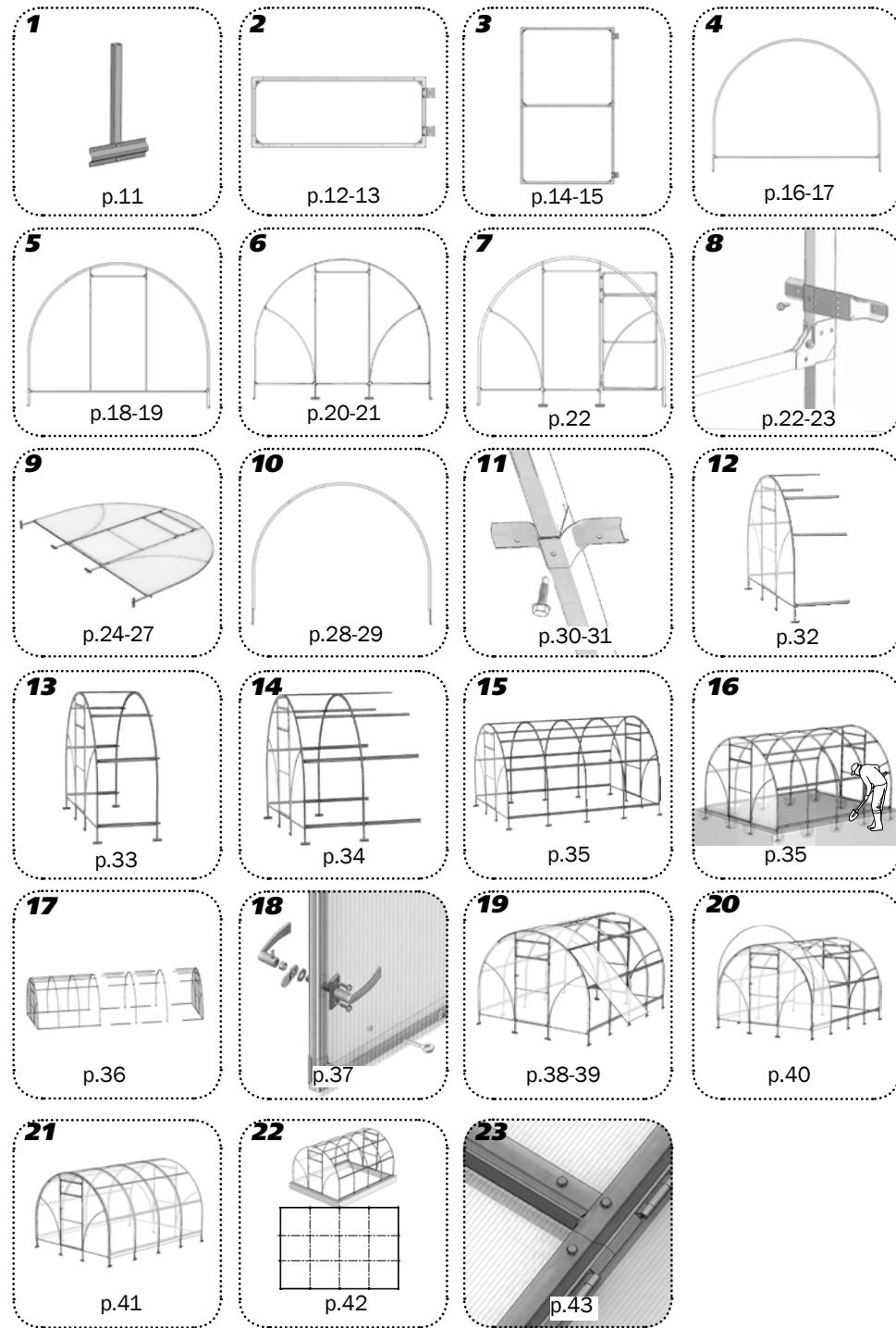
**1** If the greenhouse is mounted on a foundation (see para.22), the elements **1** and **3** are not assembled and are not mounted in the subsequent assembly.
