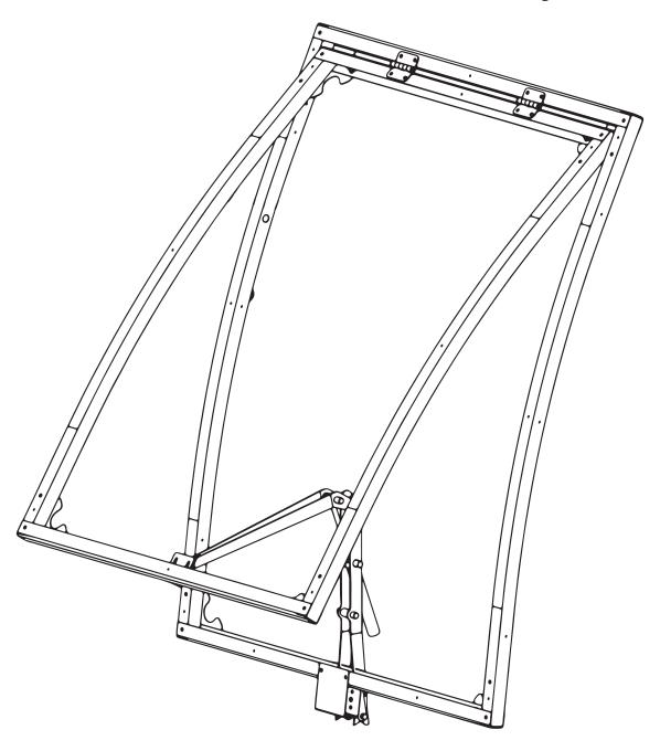
The vent for greenhouse Strong NOVA is designed to the Greenhouse ventilation and is installed in the roof of the greenhouse with self-tapping screws with a press washer and a rubber seal. Covered with cellular polycarbonate.
