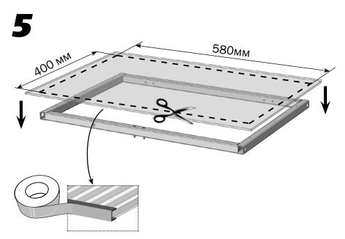
Tape scotch on the cut sides of the polycarbonate sheets.
